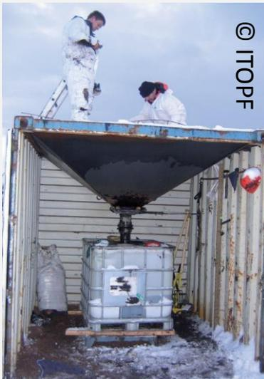
**Makeshift system to separate oil from debris**
