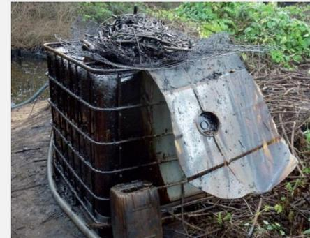
**Makeshift dripping system to separate tree branches from liquid oil**
