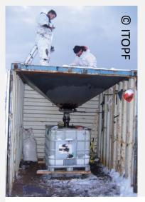
Makeshift system to separate oil from debris
