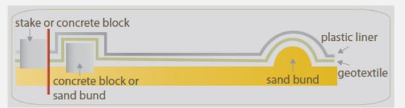
Sectional view of a watertight platform with an outer edge made of earth or concrete blocks to contain rainwater
