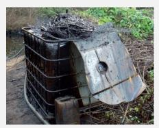
Makeshift dripping system to separate tree branches from liquid **Oil**
