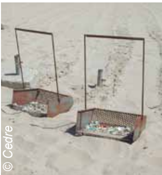
Small baskets made of meshing used to recover solid debris
