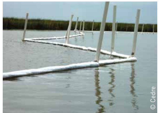
Herringbone configuration (on each side of the river)
